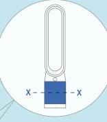
Activated carbon filter An internal network of microscopic pores mean the activated carbon in this filter has a surface area the size of 40 football pitches.
